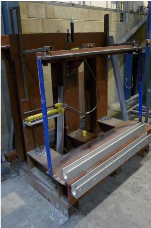
Figure 1 Strongback prior to glass installation
