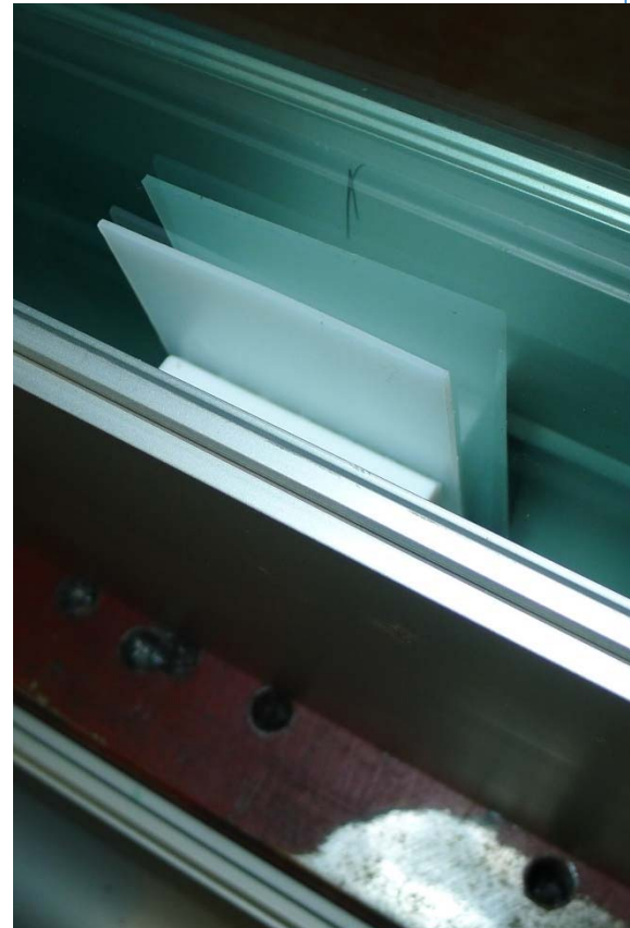
Figure 4 Shim for monolithic panels in situ, prior to fixing in position with the top section of the clamp.
