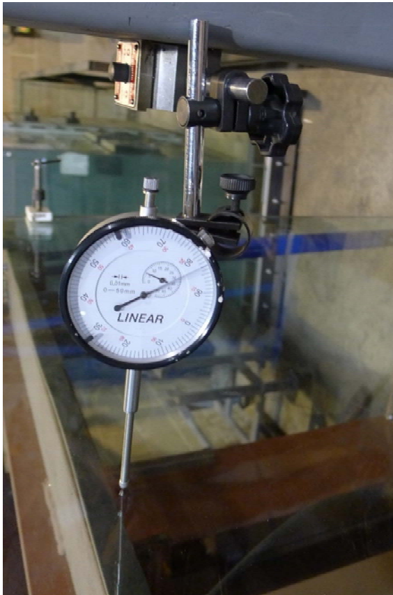
Figure 5 Upper dial gauge in situ
